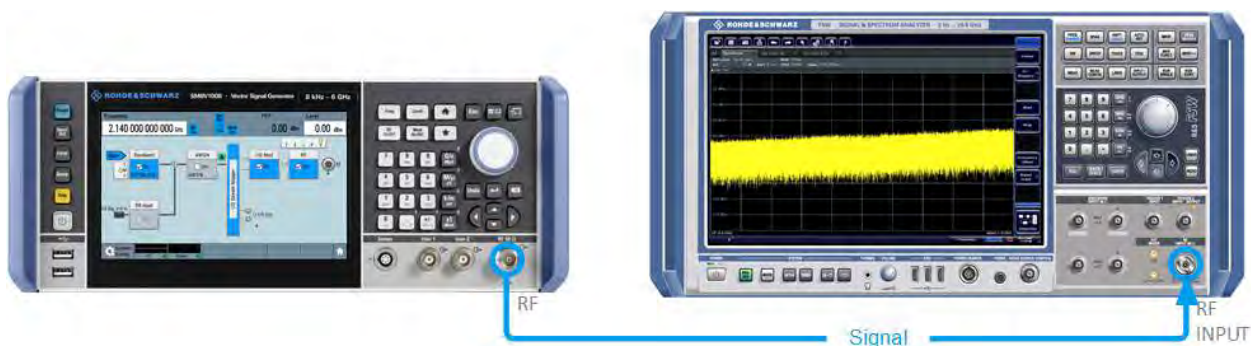
Figure 2-5: Simplified test setup
