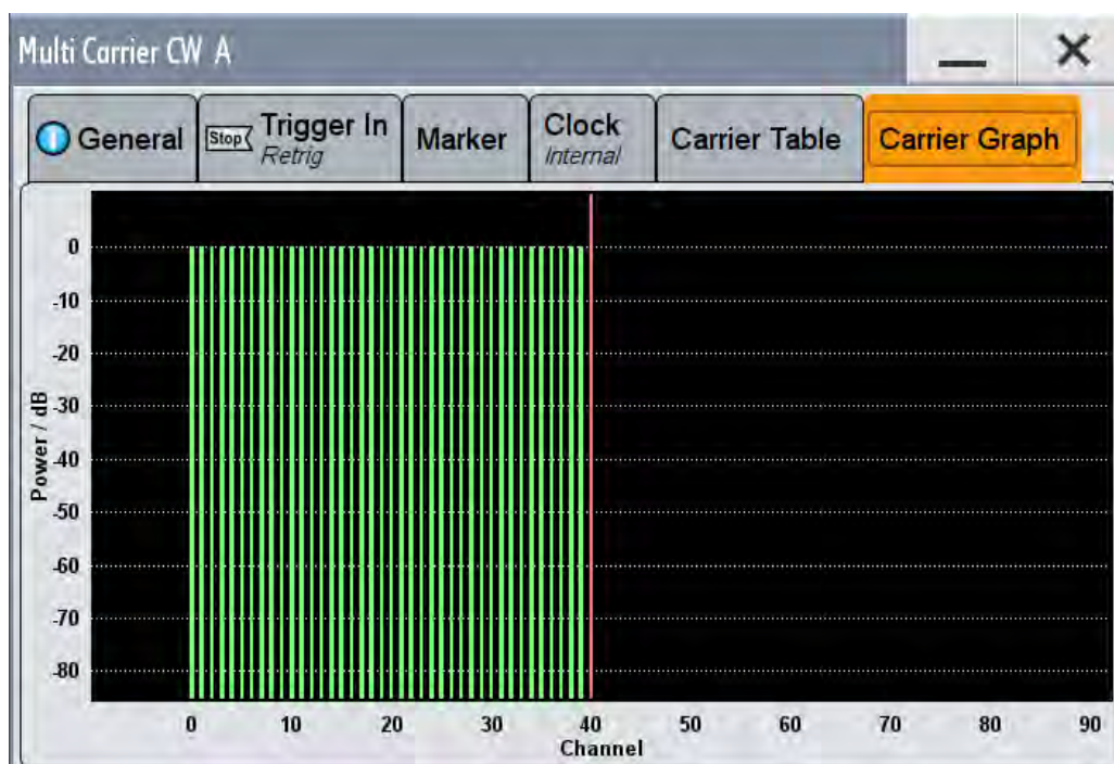
Figure 12-9: Multi-carrier signal to test the image rejection of an SSB filter
