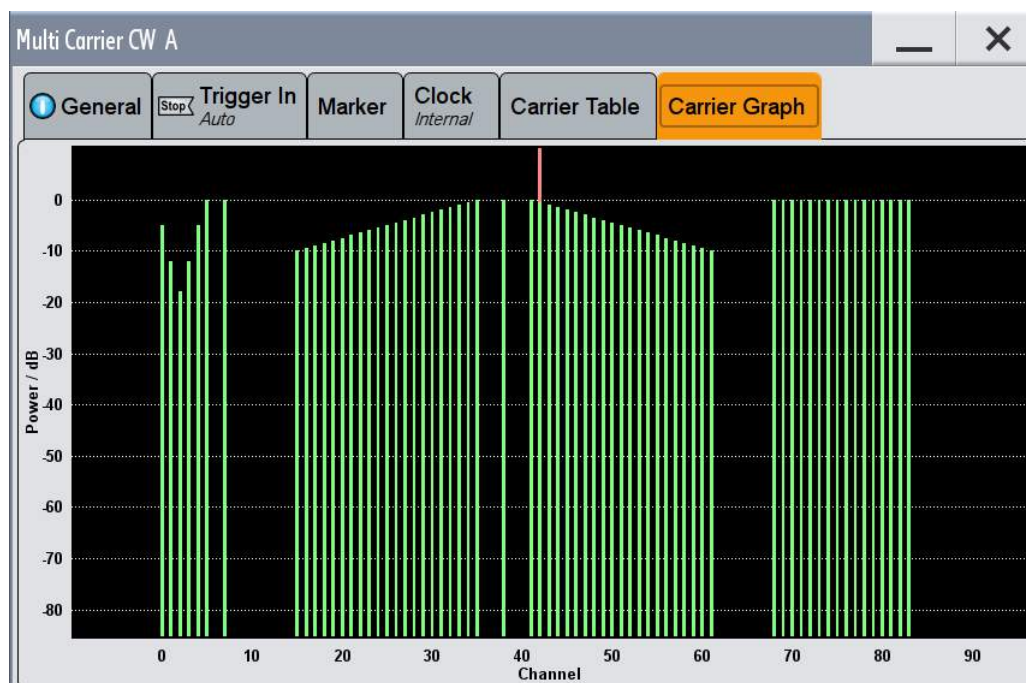
Figure 12-10: Composed multi-carrier signal
