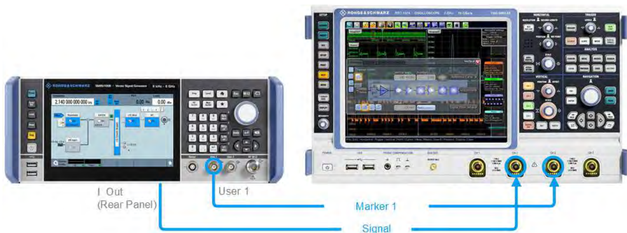
Figure 2-10: Simplified representation of a test setup for signal monitoring**
