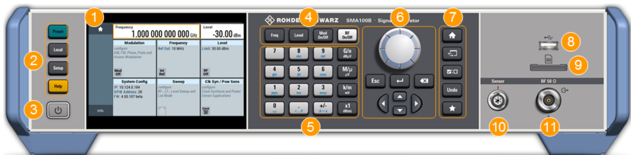
Figure 5-1: Front panel view of the R&S SMA100B RF Signal Generator with height unit 2HU (option R&S SMAB-B92)
