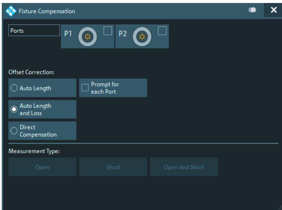
The fixture compensation menu offers a good overview of all available compensation methods.
