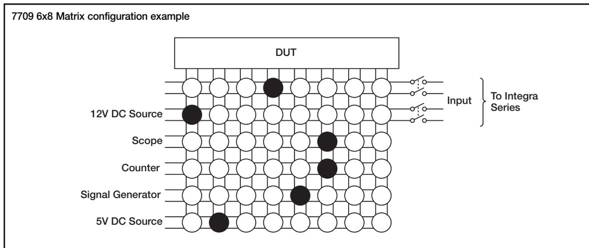
The 7709 Matrix Module can connect any combination of six differential channels of instrumentation to any combination of eight differential DUT channels. The instrumentation can be the Integra system's internal DMM or external equipment (AC and DC sources, internal or external meters, oscilloscopes, etc.) This matrix configuration allows wide flexibility for complex test systems.
