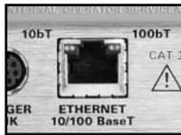
The Model 2701 offers a 10/100 BaseT Ethernet connection for high speed and long distance communication between a computer and a virtually infinite number of instruments. Any PC with an Ethernet port can connect to a single Model 2701 in a point-to-point configuration, to multiple 2701s through a hub, or to multiple 2701s distributed on a network. See the system configuration section on page 35 for more details on Ethernet connections.
