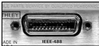
The Model 2700 and 2750 both offer a GPIB port. GPIB provides higher speed data transfers (up to 1Mbyte/sec.) than RS-232, and allows up to 32 devices to be addressed from a single GPIB controller card in a host computer. The maximum cabling distance for the GPIB interface is 2 meters between each GPIB connection. Up to 20 total meters of cable may be connected to a single controller card.
