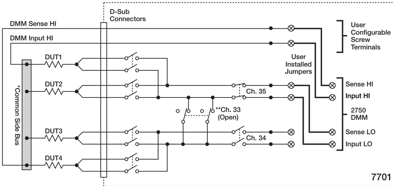
\*NOTE: Common side connections must be made carefully to eliminate all lead resistance from the 4-wire ohms measurement. The common side bus should be a single wire or bus bar that connects the HI side of all the DUTs. DMM Input HI should be connected to one end of the common side bus and DMM Sense HI should be connected to the other end.
