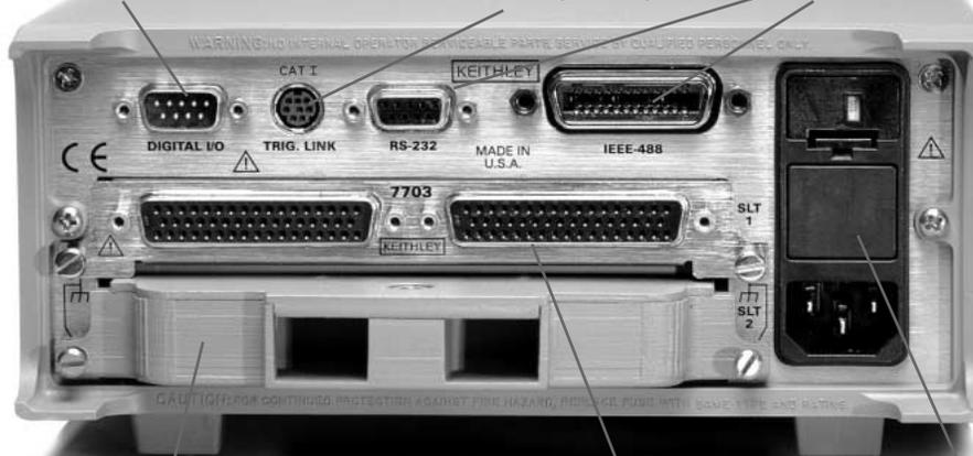
A variety of measurement and control modules let you mix, match, and change input signals or control lines any time you like. Install up to two modules at a time to create up to an 80-channel "mini-ATE" system.
