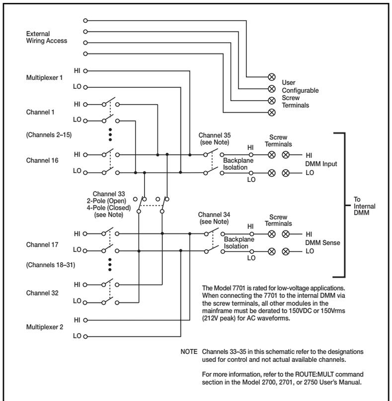
See page 43 for common-side 4-wire ohms configuration example.
