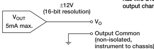
NOTE: The 7706 module has two  $\pm 12V$  analog output channels.
