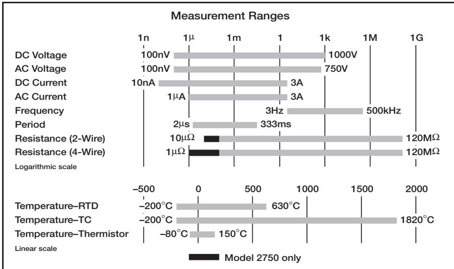
Figure 2. Measurement Ranges
