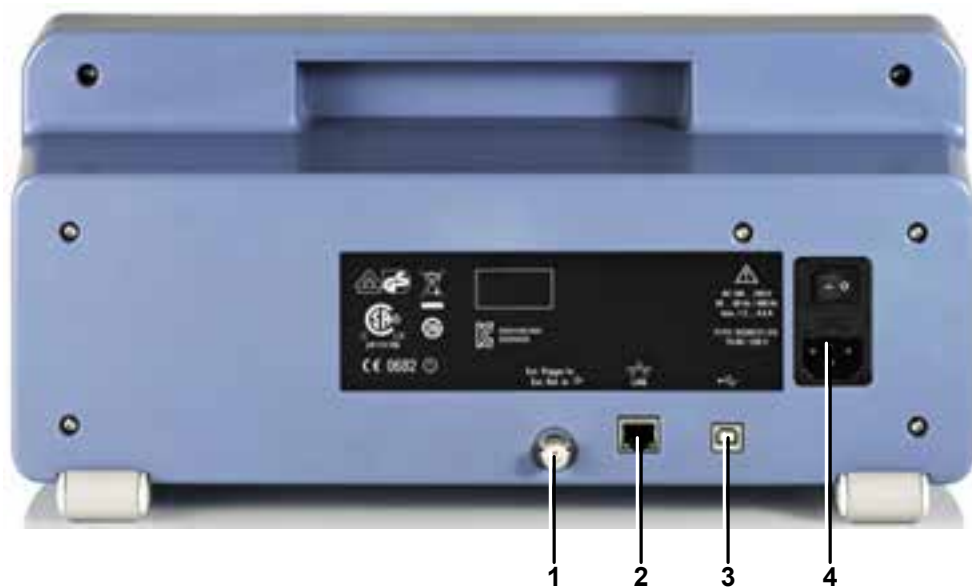
Figure 3-2: Rear panel of the R&S FPC1000
